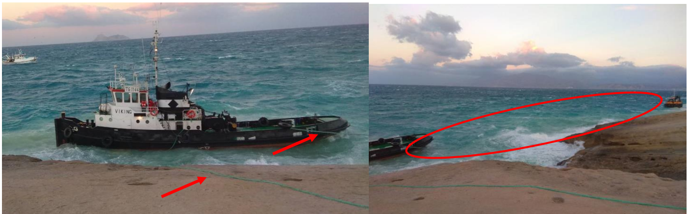
Figure 6: Captures during the grounding of VIKING; in the left image, the two lines indicated are the ones used for abandonment and the tow line, still attached to the dredger. In the right image the tow line is discerned floating (within red ellipse).
